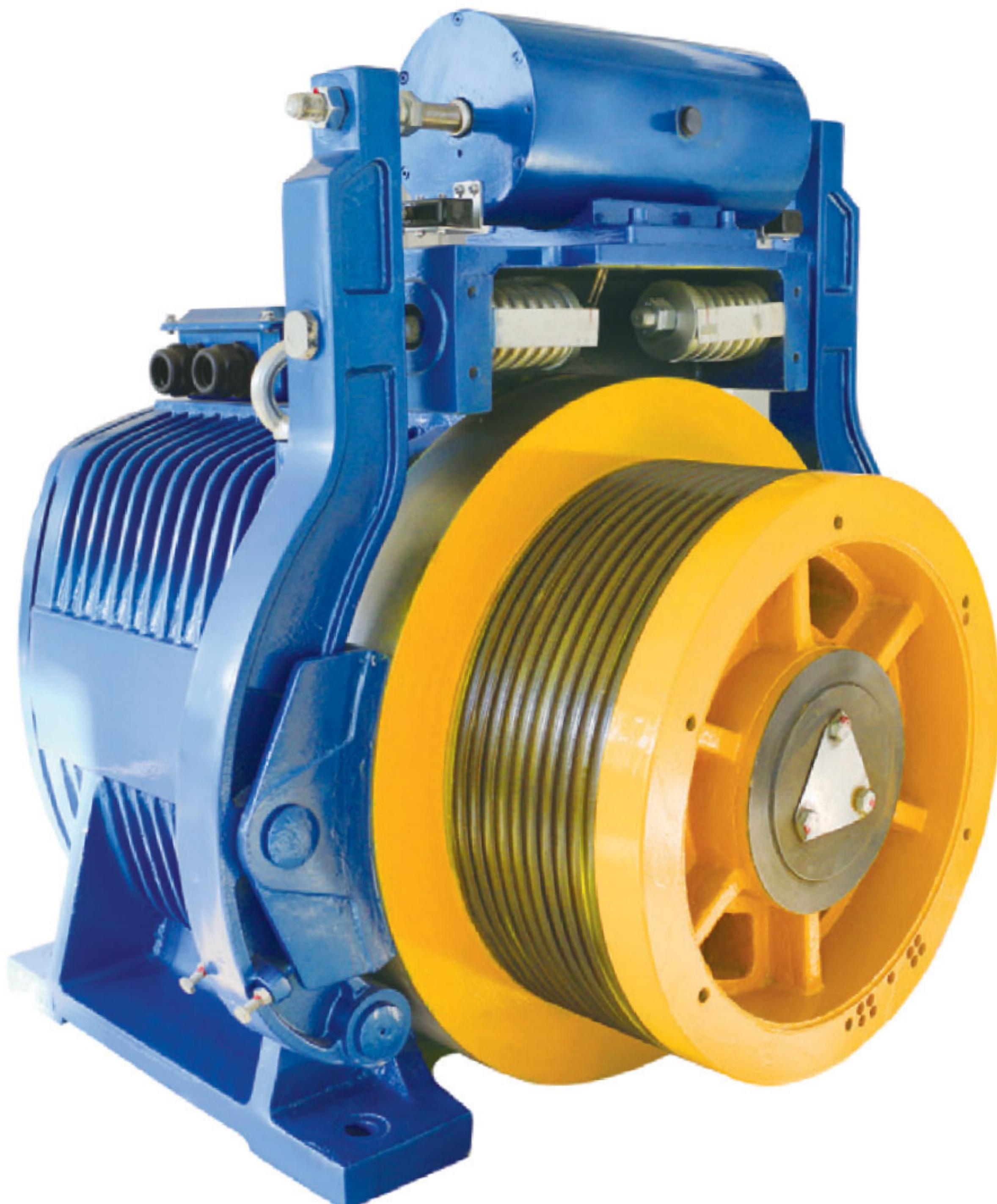
WYT-Y series inner rotor type PM gearless traction machine is developed by Bluelight in 2004 for high speed (up to 4m/s) & high capacity (up to 2000kg) elevator. After long time of improvement & optimization, this series has development second version (MK II).
